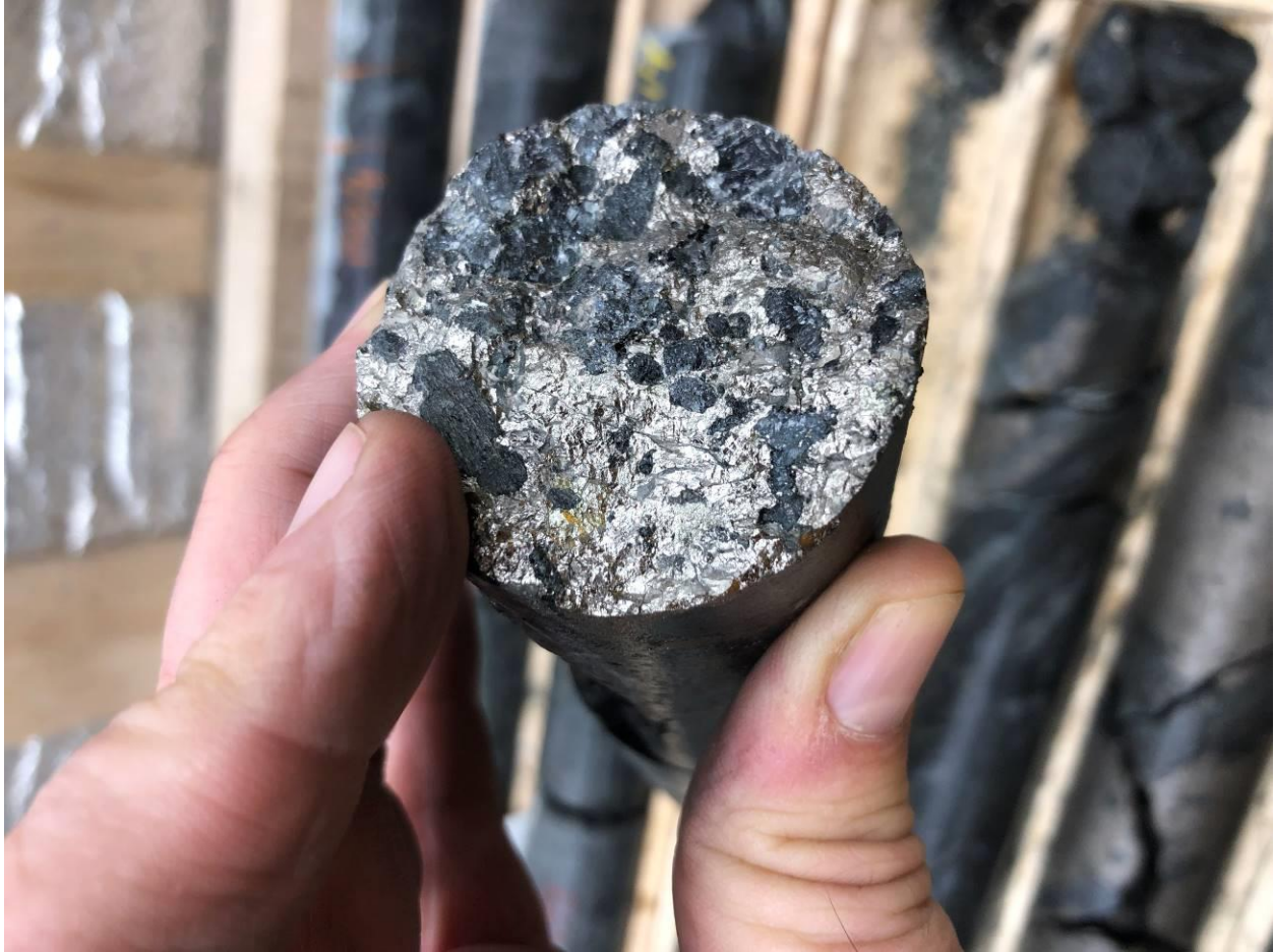
Figure 36: Mineralized core with Po & silicate or oxide inclusions during physical inspection by Claude Duplessis
