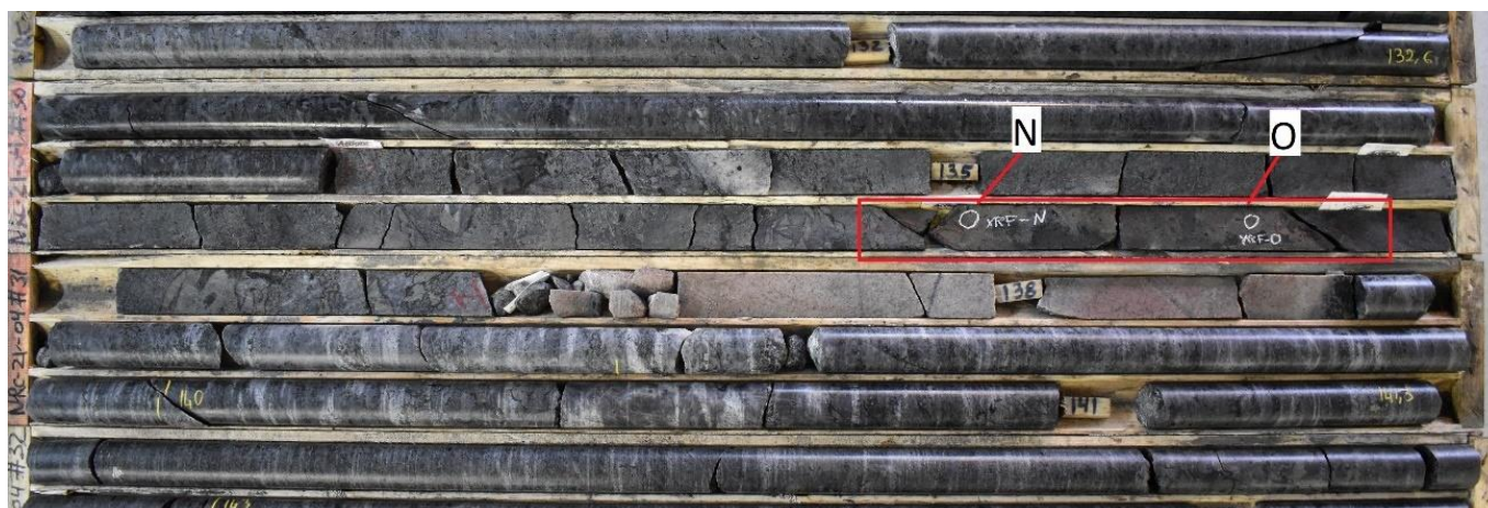
Figure 29: Core Photo of best intercept on Discovery zone within NRC-21-03 showing massive sulfide mineralization - Box 29-31 (134.70m – 147.20m)
