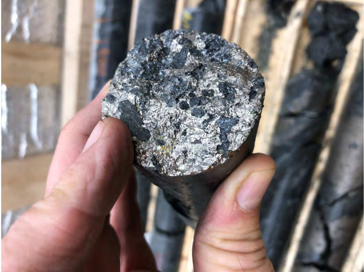
Figure 36: Mineralized core with Po & silicate or oxide inclusions during physical inspection by Claude Duplessis P. Eng.
