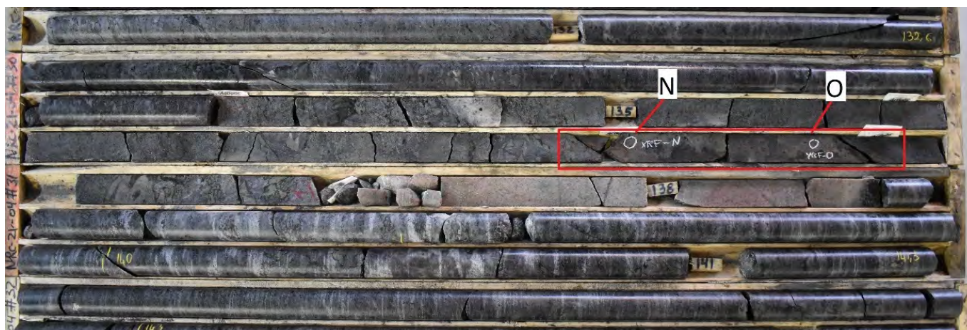
Figure 29: Core Photo of intercept on Discovery zone within NRC-21-03 showing massive sulfide mineralization - Box 29-31 (134.70m – 147.20m)
